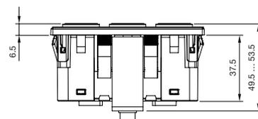
The keypad can be mounted into front plate thicknesses between 1 and 4 mm. A front plate of at least 2 mm thickness is recommended. Non-compliance with these specifications may lead to damage to the locking tongue.
