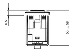
The keypad can be mounted into front plate thicknesses between 1 and 4 mm. A front plate of at least 2 mm thickness is recommended. Non-compliance with these specifications may lead to damage to the locking tongue.
