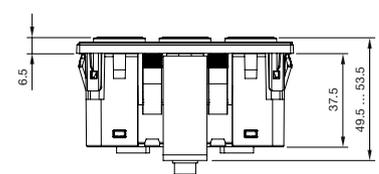
The keypad can be mounted into front plate thicknesses between 1 and 4 mm. A front plate of at least 2 mm thickness is recommended. Non-compliance with these specifications may lead to damage to the locking tongue.
