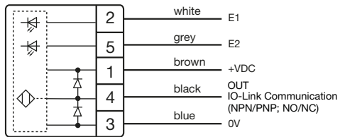
Connection plan 5-pin
