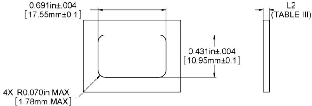
Figure 9: Panel cutout and thickness
