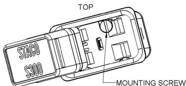
Figure 17: Mounting screw location (splash-proof version shown)
