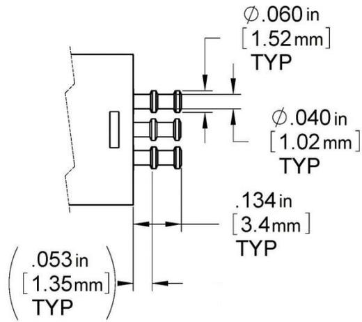
Figure 6: Solder termination
