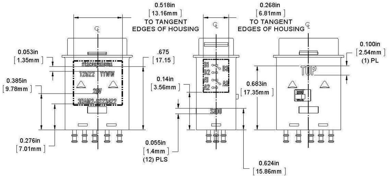
Figure 28: Marking (2 pole & Solder version shown)
