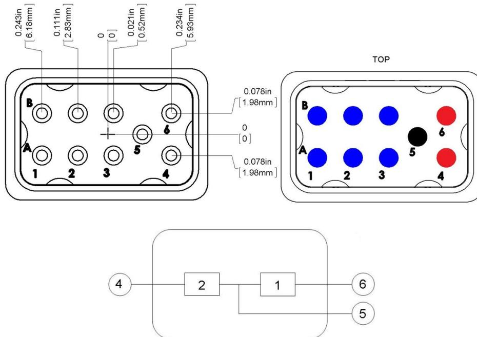
Figure 18: Switch terminal identification (28VDC Common shown)
