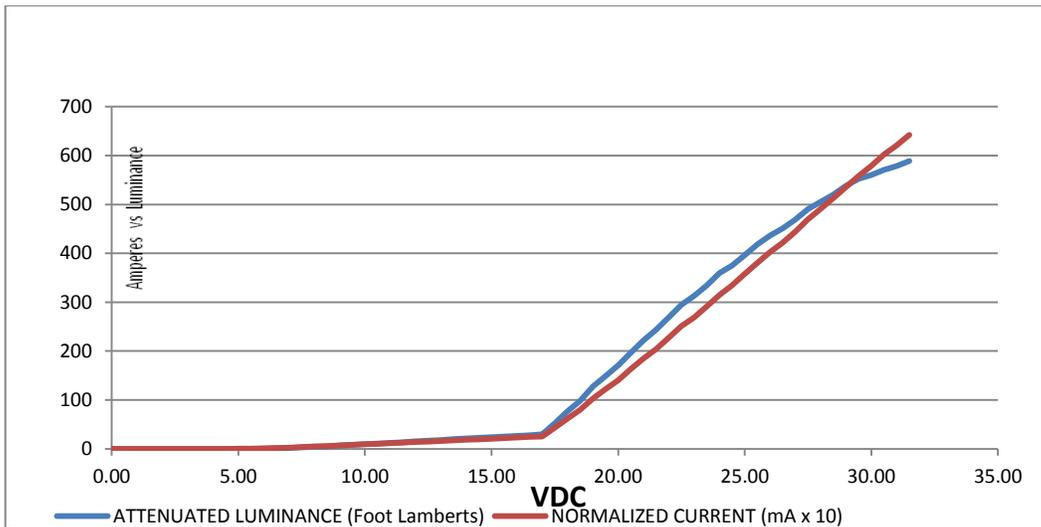
Figure 25: Typical Luminance vs Voltage (non-linear dimming)
