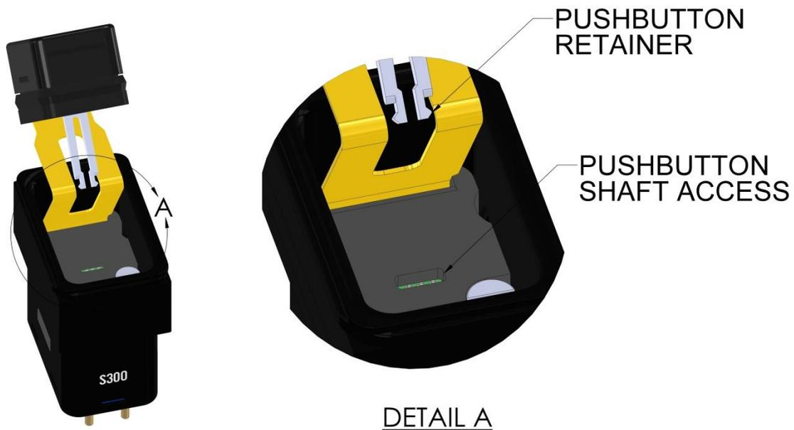
Figure 4: Detail A: Locking mechanism (drip-proof version shown)
