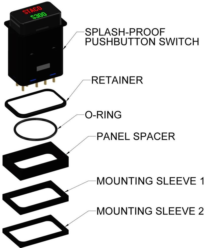
Figure 3: Drip Proof (PCB termination version shown)
