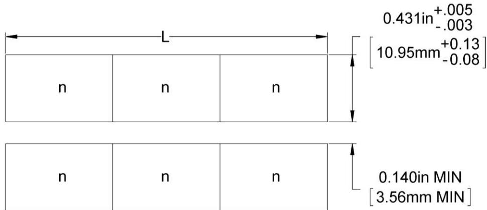
Figure 10: Slot mount for type I & III
