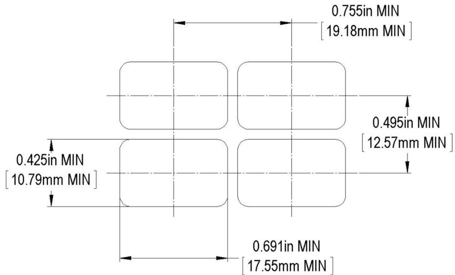
Figure 11: Matrix mount for type I & III
