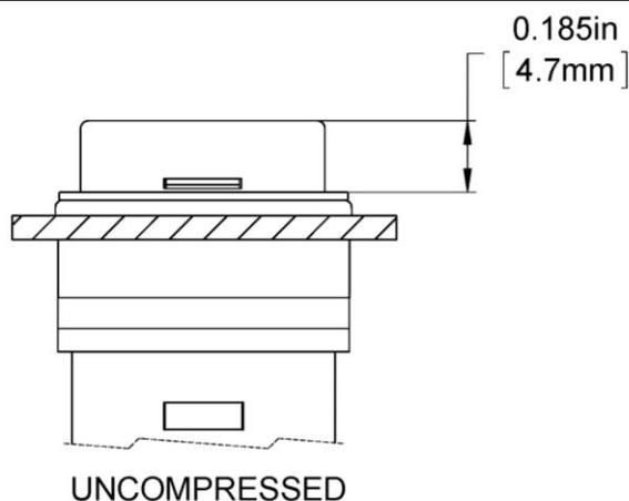
Figure 14: Pushbutton displacement for splash-proof switches (uncompressed)
