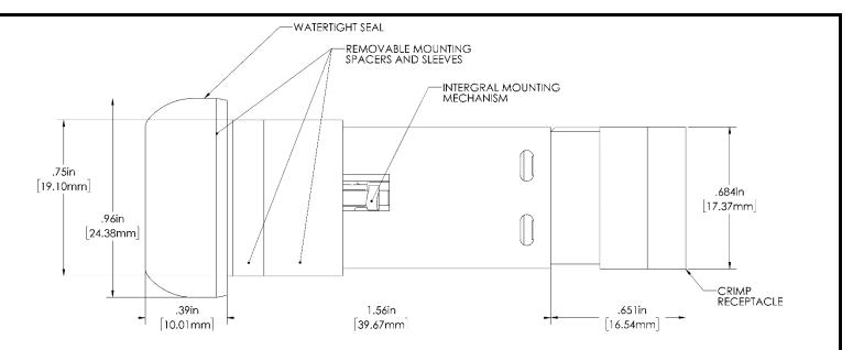
Figure 18: Splash-Proof/Watertight switches – Enclosure Type VI crimp termination (top view)
