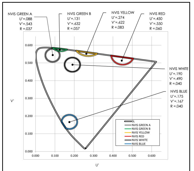
Figure 45: NVIS Compatible Colors – CIE 1976 Chromaticity Diagram
