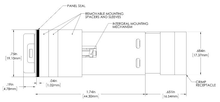
Figure 13: Drip-proof switches – Enclosure Type V crimp pin termination (side view)
