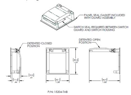
Figure 53: Pushbutton Guard for Watertight Sealed Assembly
