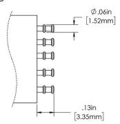
Figure 19: Solder termination
