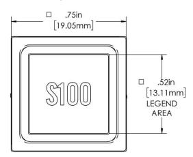
Figure 9: Drip-Proof – Solder/PCB and Crimp switches – Enclosure Type II solder and PCB termination and Enclosure Type V crimp termination (front view)
