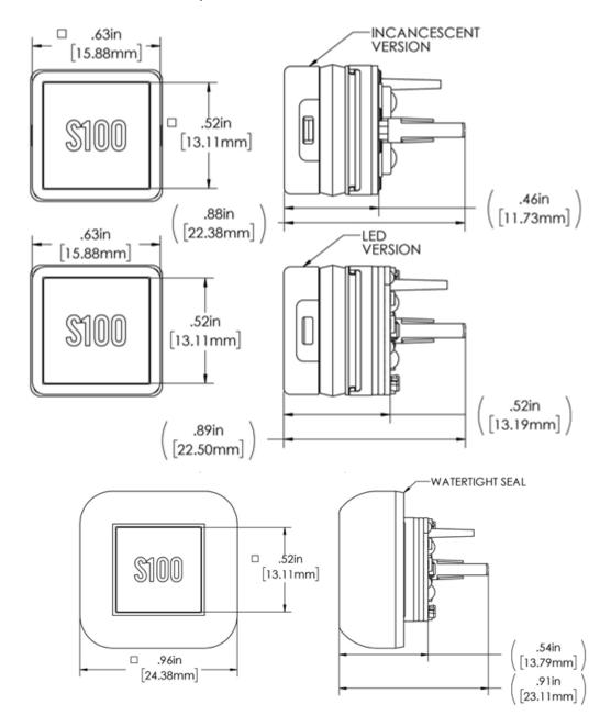
Figure 27: Pushbutton Assembly types (Incandescent/LED)
