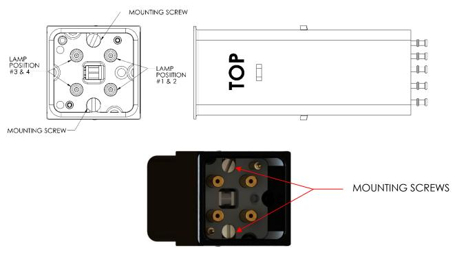
Figure 39: Mounting Provision (solder termination shown)
