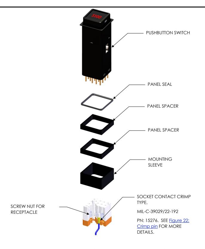
Figure 7: \$100 exploded view (Crimp termination version shown)
