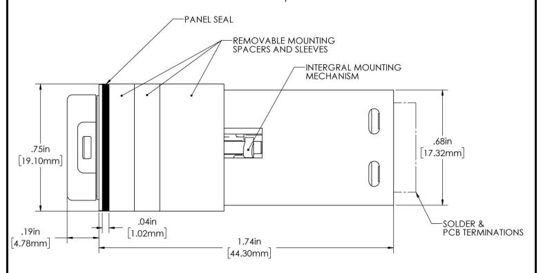
Figure 11: Drip-Proof – Solder/PCB switches – Enclosure Type II solder and PCB termination (side view)
