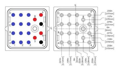
Figure 40: Switch terminal identification
