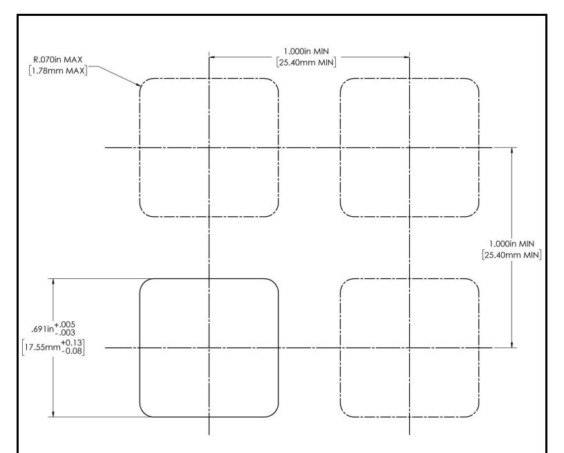
Figure 30: Matrix mount for type III & VI
