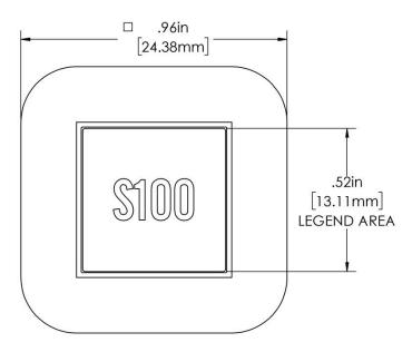
Figure 14: Splash-Proof/ Watertight switches – Enclosure Type III solder and PCB terminations and Enclosure Type VI crimp termination (front view)
