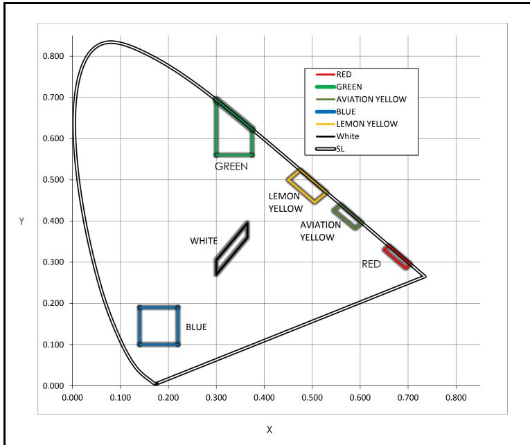
Figure 43: High Brightness LED Colors – CIE 1931 Chromaticity Diagram
