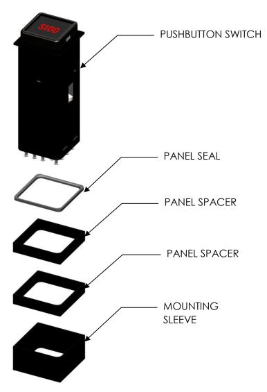
Figure 5: \$100 exploded view (solder termination version shown)
