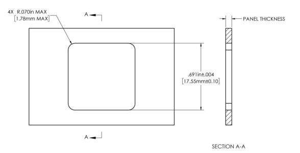
Figure 28: Panel cutout and thickness
