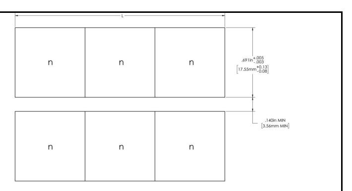
Figure 31: Slot mount for type I & III
