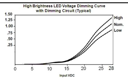
Figure 44: Voltage Dimming Curve
