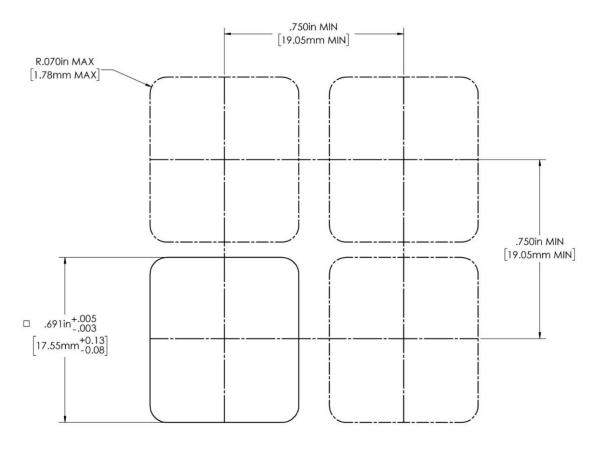
Figure 29: Matrix mount for type II & VI
