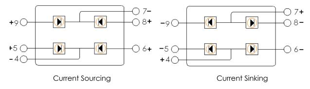
Figure 41: Pushbutton LED Polarity
