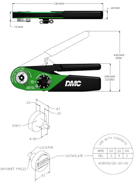
Figure 59: Crimping Pin Tools and Positioner
