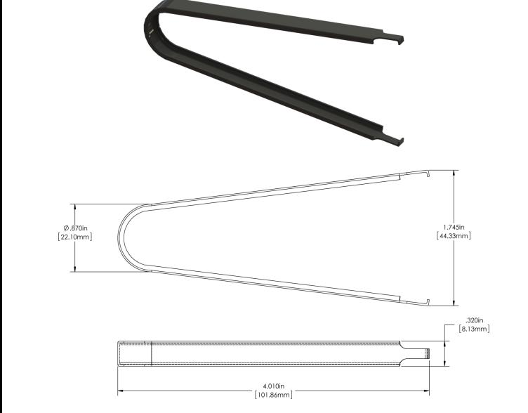
Figure 57: Pushbutton Extraction Tool
