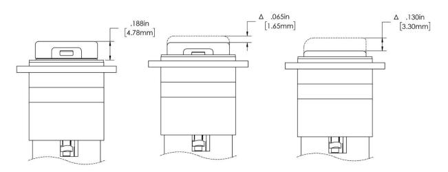
Figure 38: Pushbutton displacement for splash-proof switches
