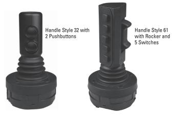
The JHM series Medium Hall Effect Joystick is a full function operator control that will fit in an armrest, on a panel, or any other location where a shallow behind panel depth joystick is needed. It utilizes Hall effect technology for long life and reliability. Electronics are sealed up to IP68S with an operational life of ten million cycles in all directions.
