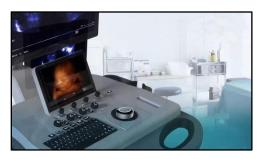
On this ultrasound panel, a Touch Encoder replaced four switches, a trackball and eight buttons.
