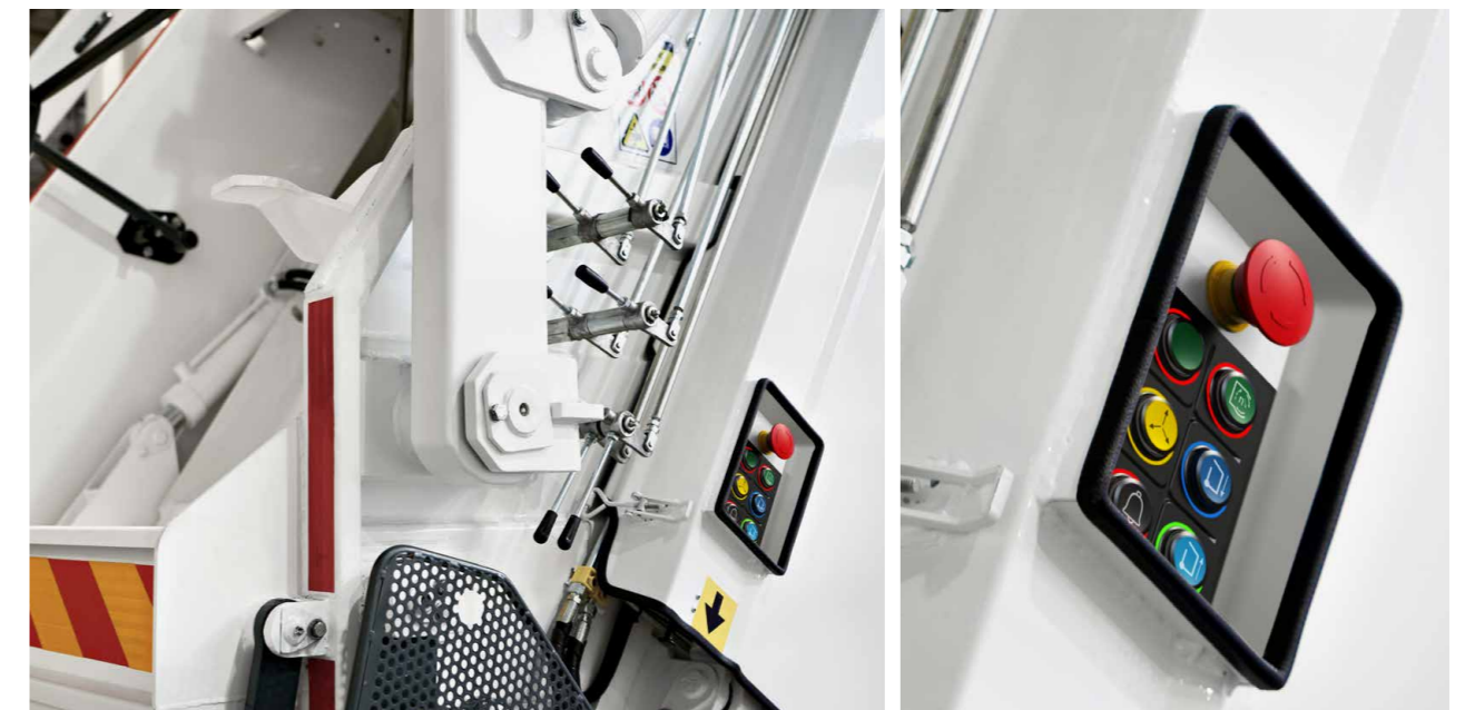
Left: Typical HMI use in a refuse truck. Right: Refuse truck panel with Series 09 and 61 HMIs.
