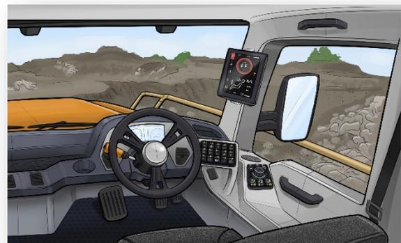
**Figure 1** Grayhill's Displays, Keypads, and MMI Controllers used on Off-highway Vehicles
