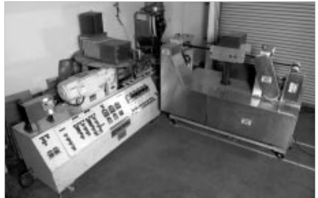
▲ Thermoplastic extruder for microwave absorbing thermoplastic products.
