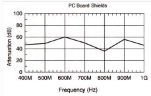
▲ Test performance in accordance with MIL-STD-285 using an aperture the same size as the 1-3/4" x 2" (44.5 mm x 5.08 mm) PC shield as reference. Measurement below 400 MHz were not possible because of the aperture attenuation.
